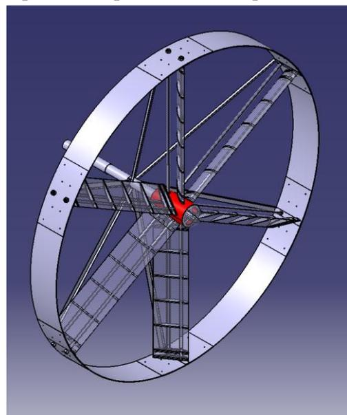
**Fig. 3. Highlighted inner cylinder of the rotor**
