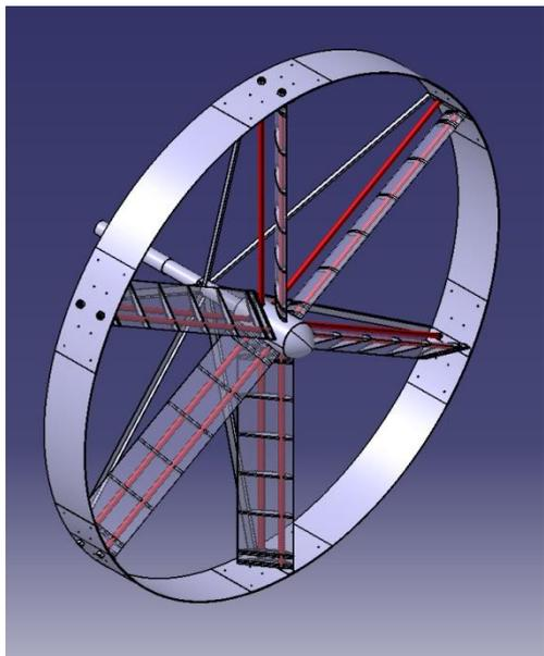
**Fig. 4. Highlighted spars of the rotor**
