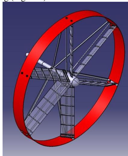
**Fig. 1. Highlighted outer ring of the rotor**
