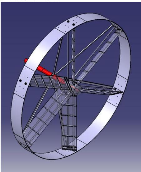
**Fig. 2. Highlighted axle of the rotor**
