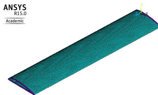
**Fig. 6. The FE model of a single blade**
