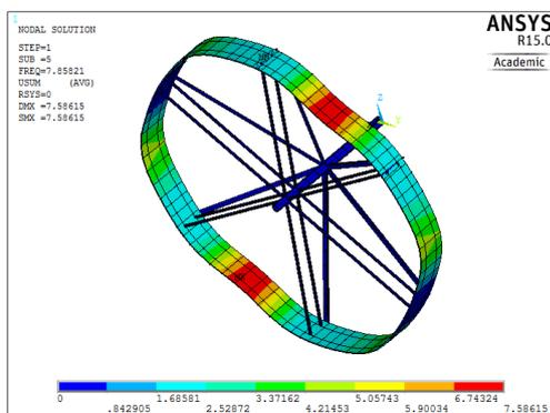
Fig. 9. Fourth mode of vibration – foam filled
